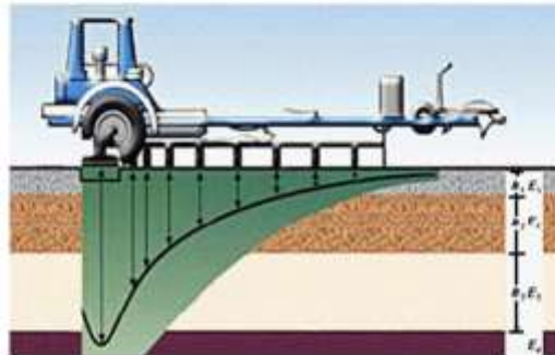
Figure 3. Schematic representation of FWD testing.
