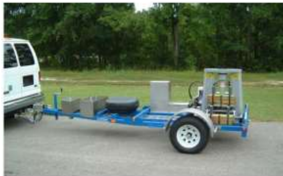
Figure 2. Dynatest 8002 FWD Test System.
