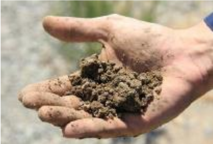
Too dry - crumbling
